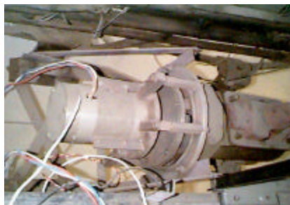
Motor which replaces the engine on a 3 wheeler
